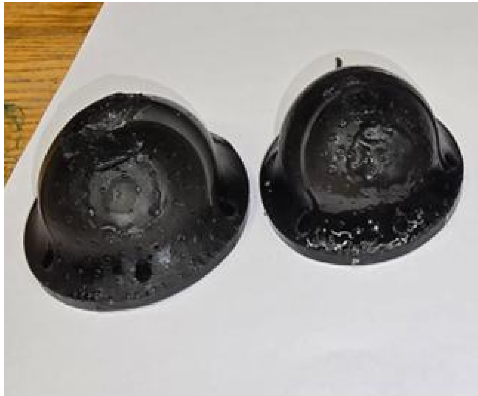
Figure 3.3: Post-curing defects observed after UV curing.
