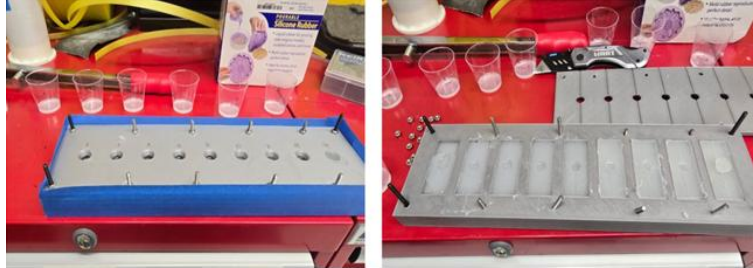
Figure 3.1: Mold used to evaluate different stoichiometric ratios of two-part silicone.
