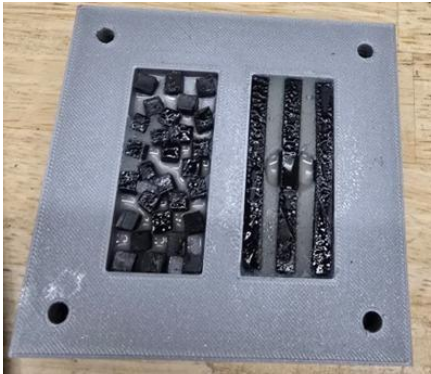
Figure 5.1: Conceptual configurations using F80 inclusions and aligned reinforcing strips for stiffness tailoring.
