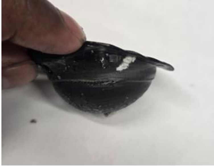
Figure 3.4: Printing defects observed during resin-based manufacturing.
