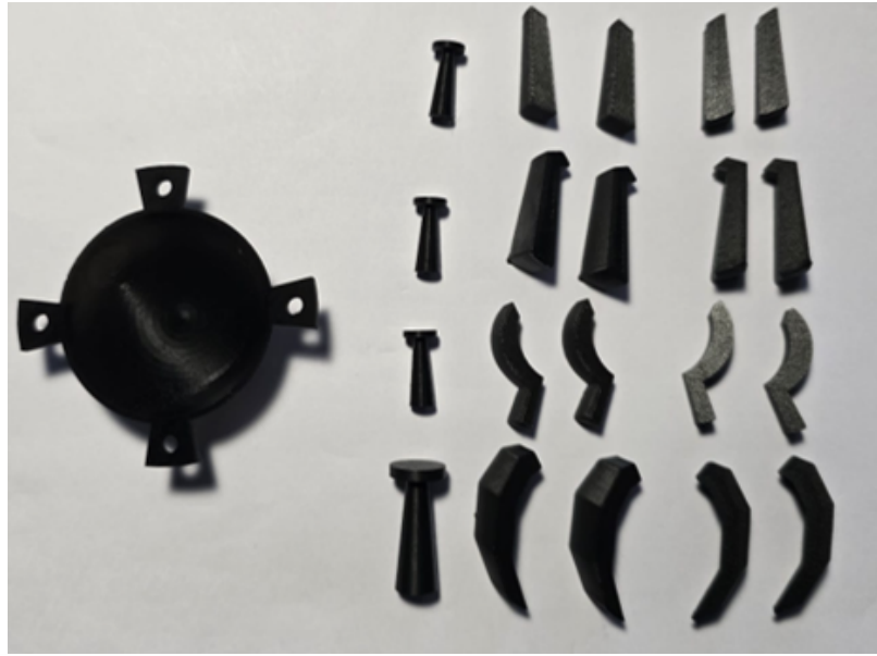
Figure 4.17: Iteration 6 shell prior to bonding, with gripper prongs and contact pad unglued.
