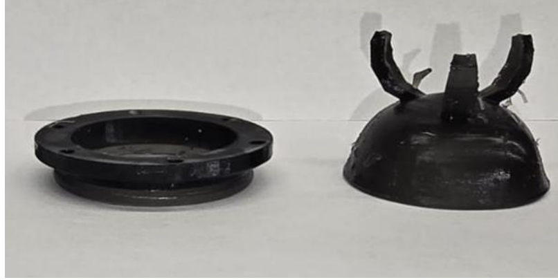
Figure 4.6: Shearing of the rim and bistable shell in Iteration 3 due to stress-concentration points along the flexure.
